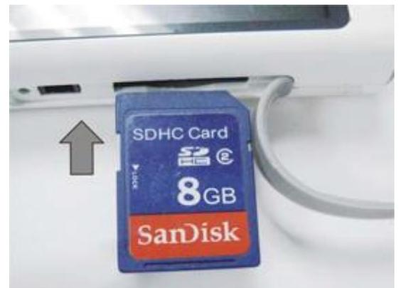
Figure 2-2 Insert SD Card
